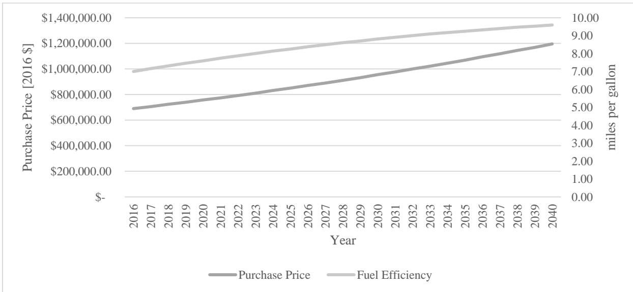
Figure 4.3 Hybrid-Diesel Bus Purchase Price and Fuel Efficiency Projection
