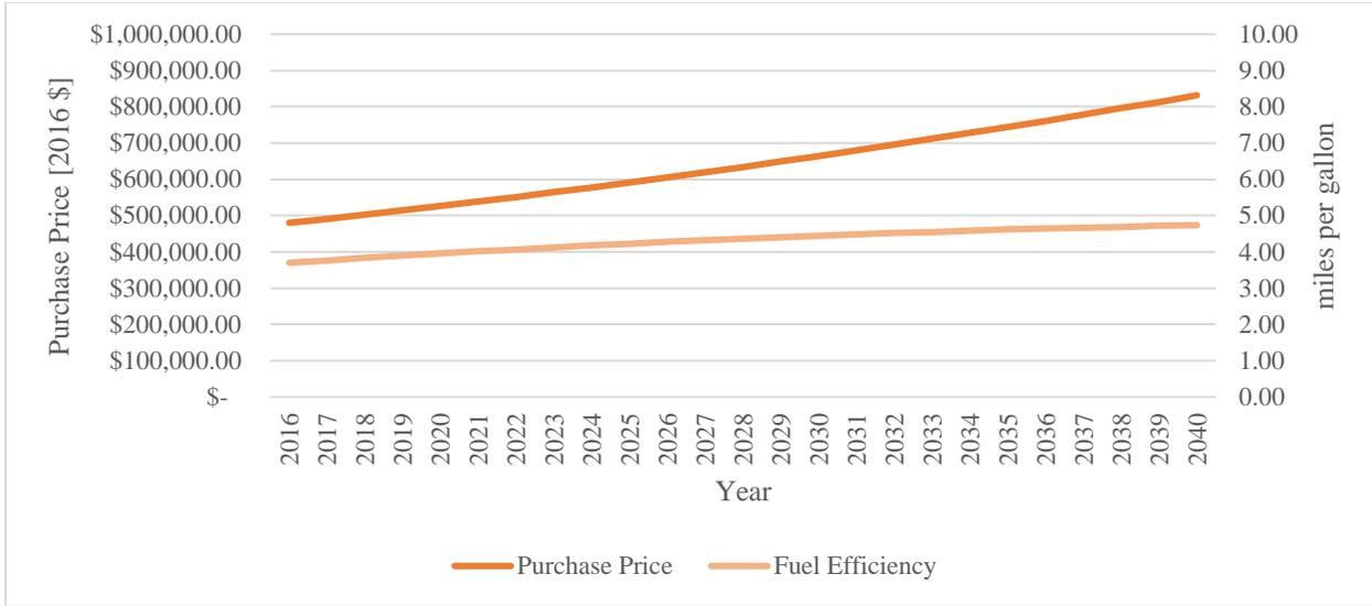
Figure 4.2 Diesel Bus Purchase Price and Efficiency Projection
